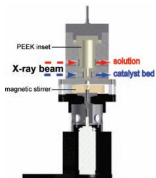
Figure 1. Schematic design of the reactor used for the QEXAFS in situ study. The two beam paths allow separate monitoring of the supported catalyst in the catalyst bed (lower window) and soluble species in the liquid phase (upper window).
